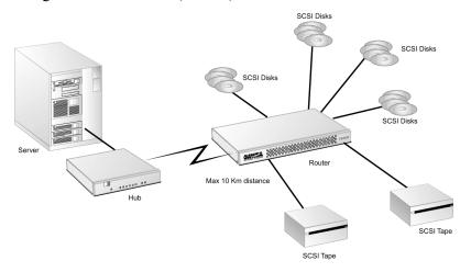
Figure 2-6. Single server configuration example
